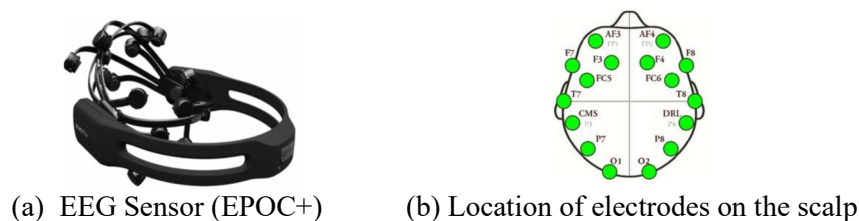
Figure 2. EEG Sensor and Location of Electrodes
