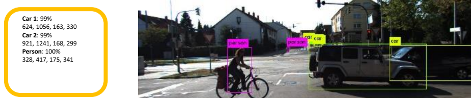
Figure 4. Image detection results in running YOLOv3 algorithms
