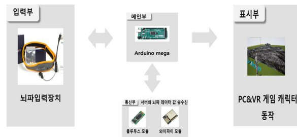
Fig. 1. Diagram of Brainwave VR controller System
