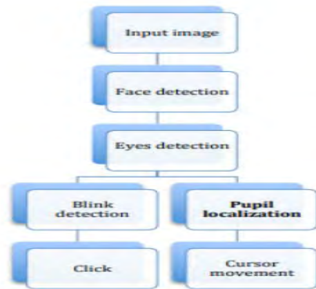
그림 3. General scheme of an image processing sequence used for eye driven computer control.
