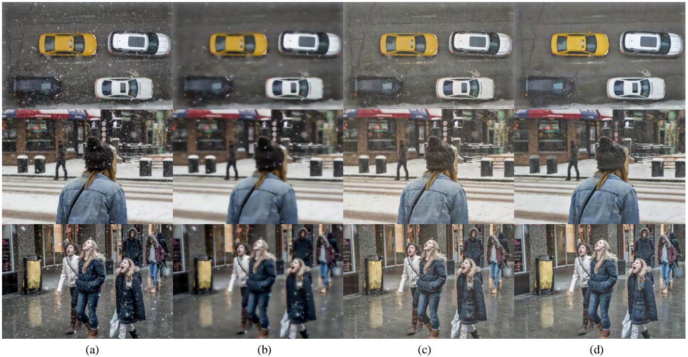
Fig. 6. Snow removal results of various methods for realistic snowy images. (a) Input image. (b) Zheng et al. [15]. (c) DeblurGAN [10]. (d) The proposed method. Best viewed on screen.
