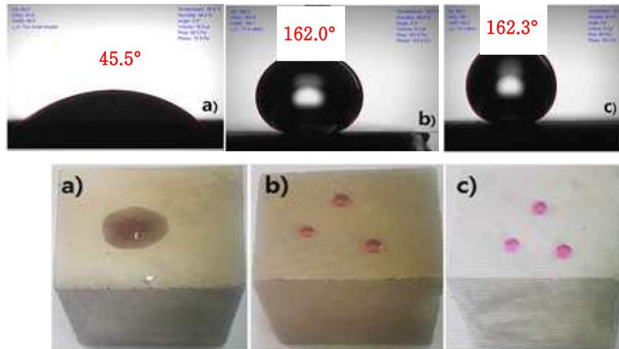
Figure 1. The contact angle measurement of normal (a), admixed (b) and coated cement mortar (c)
