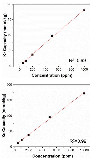
Fig. 1. Adsorption capacities at various Kr and Xe concentrations.
