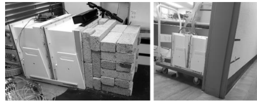
Fig. 1. Experimental setup for the experiment using a stack of bricks (left) and a building wall (right).
