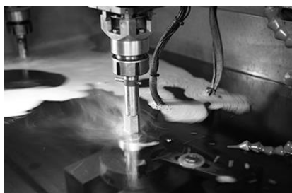
Fig. 5. Specimen taking by EDM.
