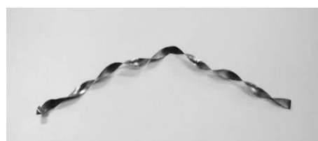
Fig. 2. Chips specimen by normal drilling.
