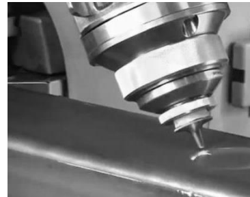
Fig. 6. Laser slope cutting.
