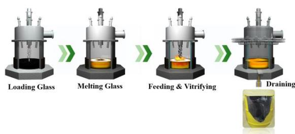
Fig. 1. Vitrification process by using CCIM [2].
