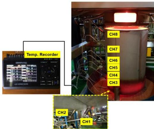
Fig. 2. Temperature recording system for the glass mold.
