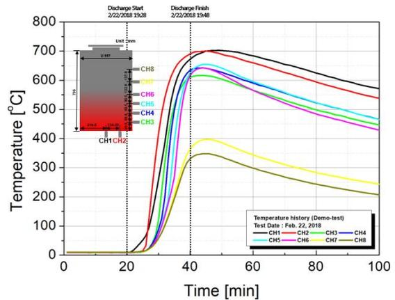
Fig. 4. Temperature history of mold for glass discharge.
