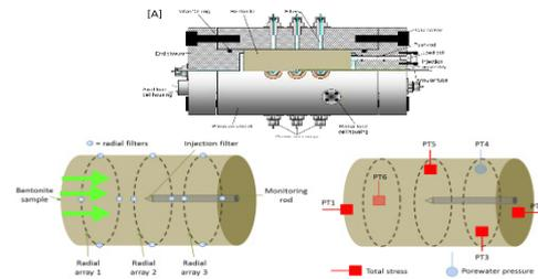
Fig. 1. Schematic view of 1D gas injection experiment [3].
