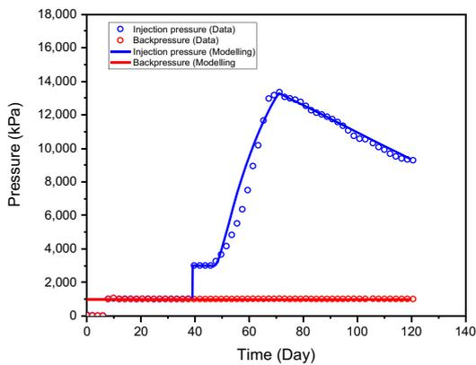
Fig. 2. Pore pressure evolution at injection filter and back pressure filter.
