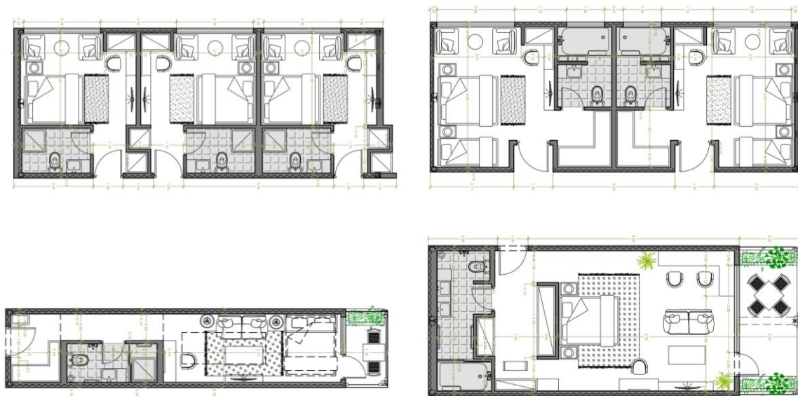
Fig.20. Room types using 40ft cargo containers
