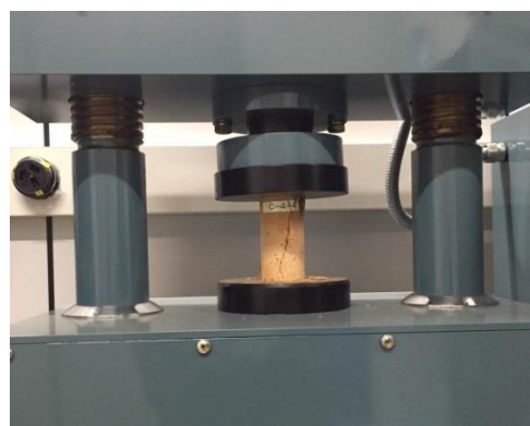
Fig. 1. Measurement of compressive strength.
