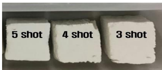
Fig. 2. Spray coated 17UD samples \text{Al}_2\text{O}_3 after drying.
