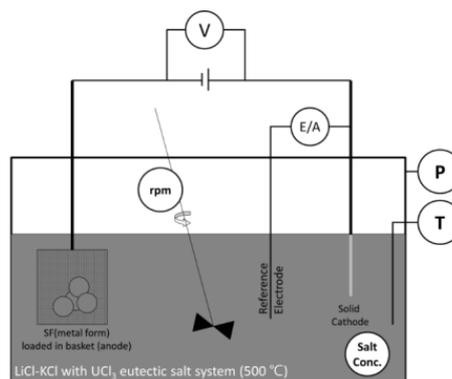
Fig. 1. Application of applicable sensors to electro-refiner.
