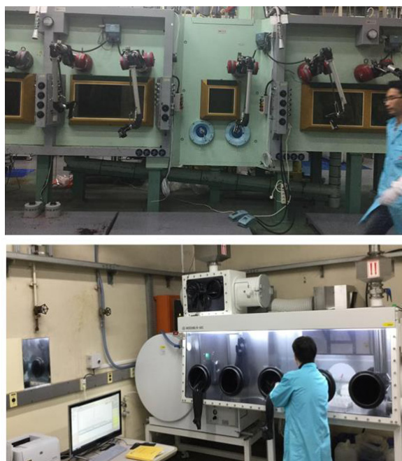
Fig. 1. Chemical hot cells (upper) and a shielded ACP-AES system (bottom).
