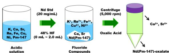
Fig. 1. Schematic illustration of Pm-147 chemical separation process.
