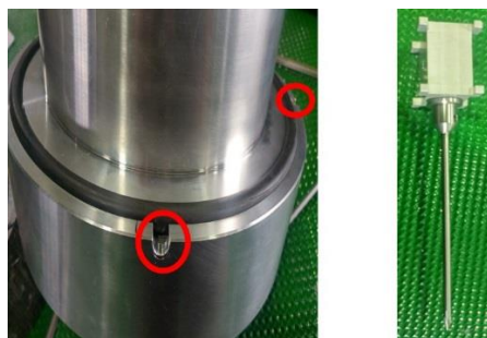
Fig. 2. O-ring holes and changing tool.
