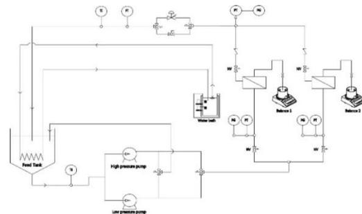
Fig. 1. Schematic diagram of the nanofiltration system. (TI: temperature indicator, FT: flow transmitter, PT: pressure transmitter, PG: pressure gauge, and NV: needle valve)
