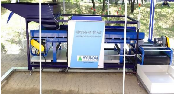
Fig. 2. Real-time measurement and segregation system.
