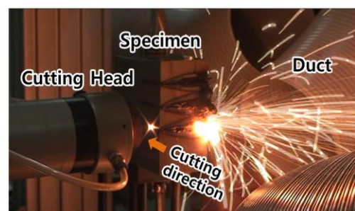
Fig. 1. View of the laser cutting experiment. The cutting started from the side of the specimen and proceeded with the cutting head moving from the right to the left.
