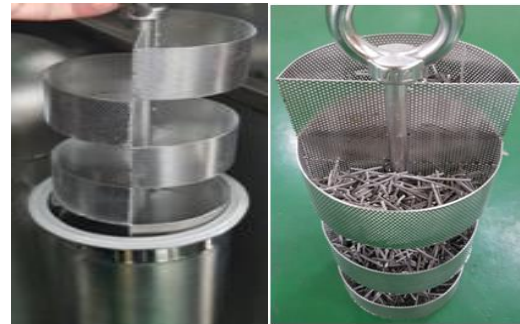
Fig. 4. Image of the interior of the adsorption tower.
