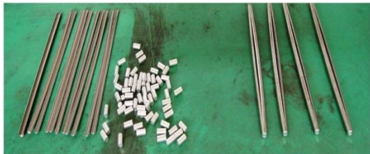
Fig. 5. Slitting shapes of 2-CUT and 3-CUT modules.
