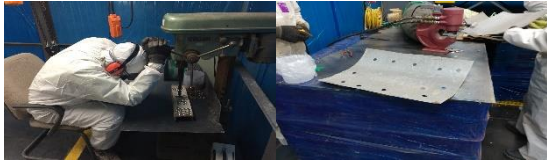
Fig. 2. Punching and Drilling of Metal.
