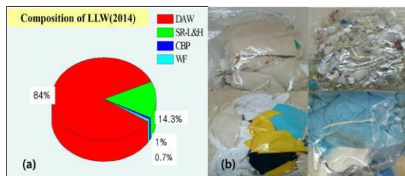
Fig. 1. Composition of low level radioactive waste from nuclear power plants in 2014 (a), and picture of dry active wastes (b).
