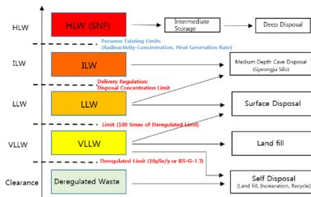
Fig. 1. Radioactive Waste Classification vs Disposal Option.
