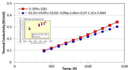
Fig. 1. Calculated and measured thermal conductivity for U-19Pu-(MA-RE)-Zr.
