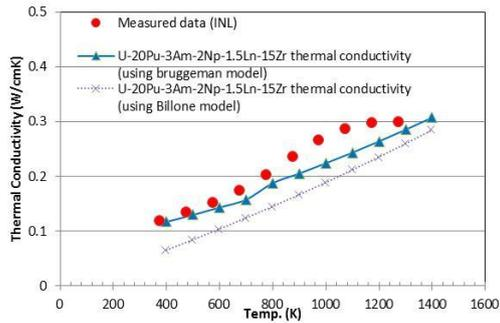
Fig. 3. Calculated and measured thermal conductivity for U-TRU-RE-Zr.
