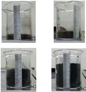
Fig. 1. Volume expansion of two samples after oxidation: packing height of 1 cm (left) and 1.5 cm (right).
