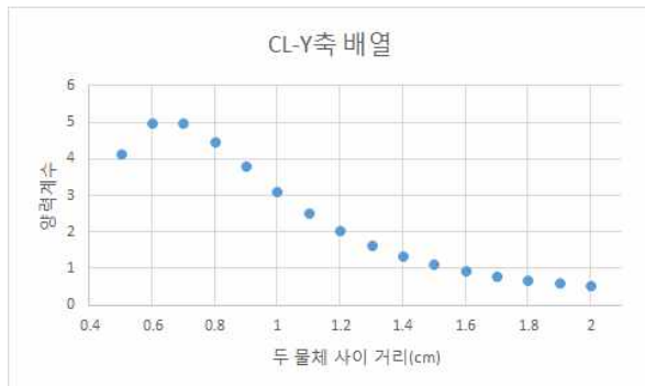
Fig.4 Coefficient of lift of vertical array
