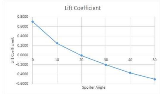
Fig. 3 Lift coefficient
