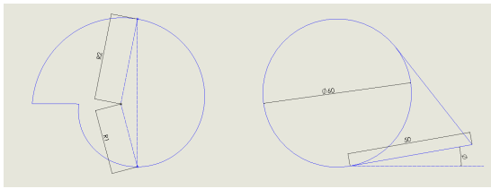
Fig. 1 Coanda flap geometry spiral(left), wedge(right)
