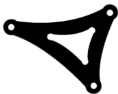
Fig. 12 The upper leg of Jansen final blueprint
