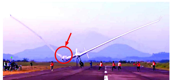
Fig. 1 Failure of human powered aircraft main Spar
