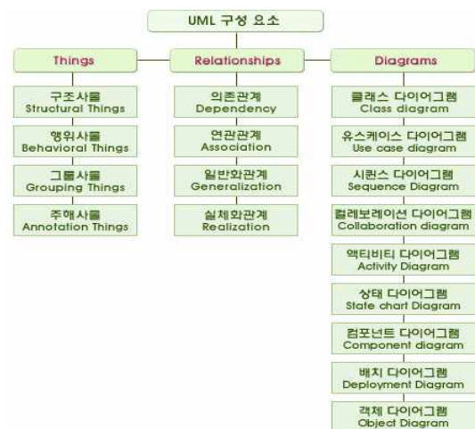
Fig. 1. Component of UML
