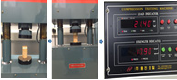
Fig. 4. Measurement of Compressive Strength.
