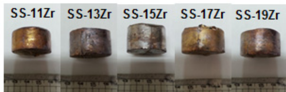
Fig. 1. Morphology of metallic waste form controlled by binary alloy element compositions.
