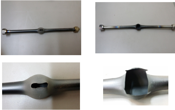
Fig. 3. Failed fuel rod by burst (rod pressure: 50atm, heating rate: 10°C/min.).
