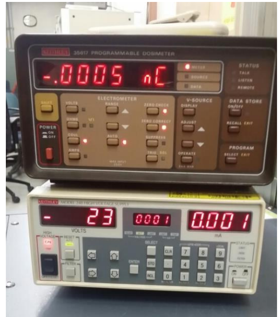
Fig. 2. Electrometer and high-voltage supply.
