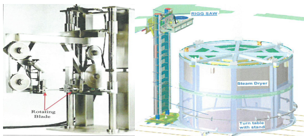
Fig. 1. Band Saw(left) & Rig Saw for Core Shroud/Steam Dryer.
