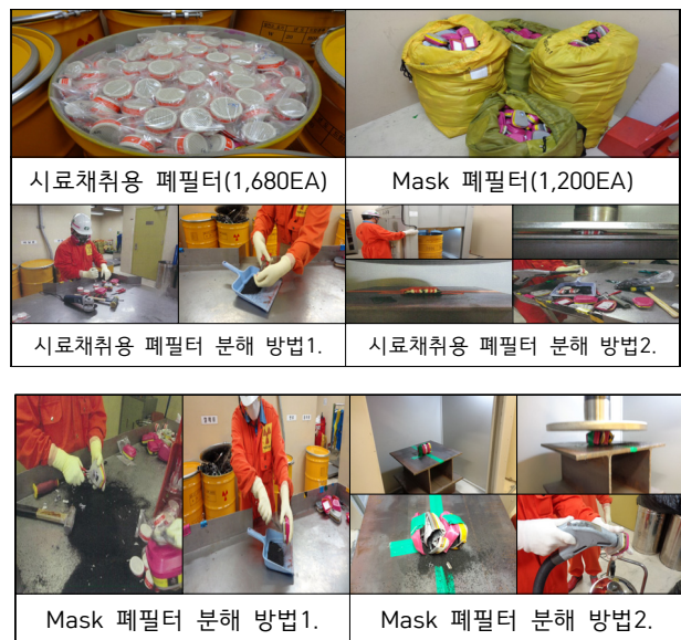
Fig. 2. Pre-improved storage and treatment Spent Charcoal filter.
