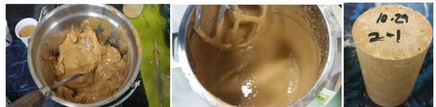
Sludge phase of radioactive waste      Mixed with solidification agent and radioactive waste      Hardened radioactive waste
