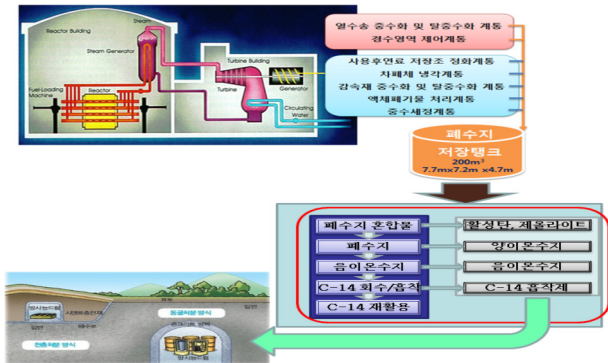
Fig. 1. Disposal of waste resin from CANDU.
