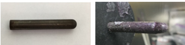
Fig. 4. Comparison of electrode surface after scraping process; Tungsten (left) and STS (right) electrodes.
