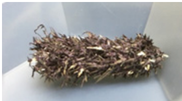
Fig. 3. Uranium dendrites scraped from Tungsten cathode.
