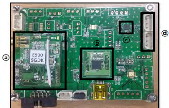
(그림 1) Capacitive pressure sensor - (a)Capacitive output, (b)Shield (c) Cover
