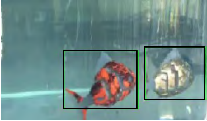
(Figure 6) Position detection of fish robots ( x_1, y_1, z_1: 82.08, 110.6, 0; x_3, y_3, z_3: 177.9, 159.7, 0 )
