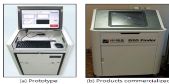
Fig. 1. apparatus for leakage detection of heavy water.
