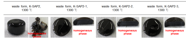
Fig. 5. Images of vitrification product with SrCl 2 and CsCl.
