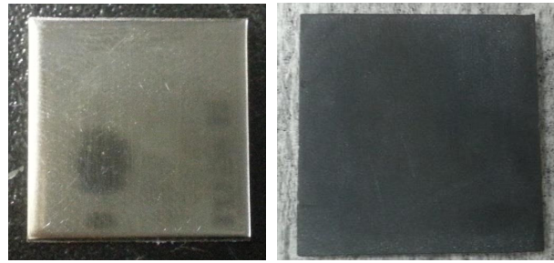
Fig. 3. Before corrosion and after corrosion of Coupons.
