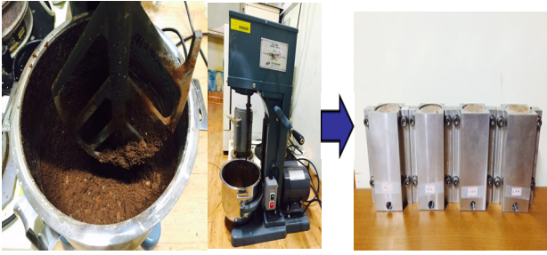
Fig. 1. The mixing process (metal oxides size : smaller than 1.4mm).
