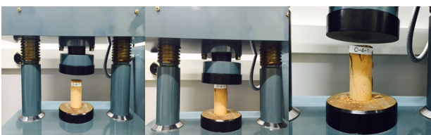
Fig. 2. Compression strength measuring process.
