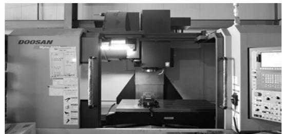
Fig. 1. Machining center (Mynx-6500).
